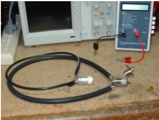
Photo C: Ferrite choke measuring loops
