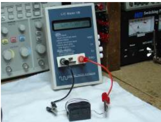
Photo A: AADE Inductance Measurement Photo B: AIM4170B Swept Measurement
